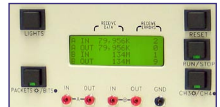
▲ Front-panel controls and test points provide access to the NTDS signal lines for detailed analysis
